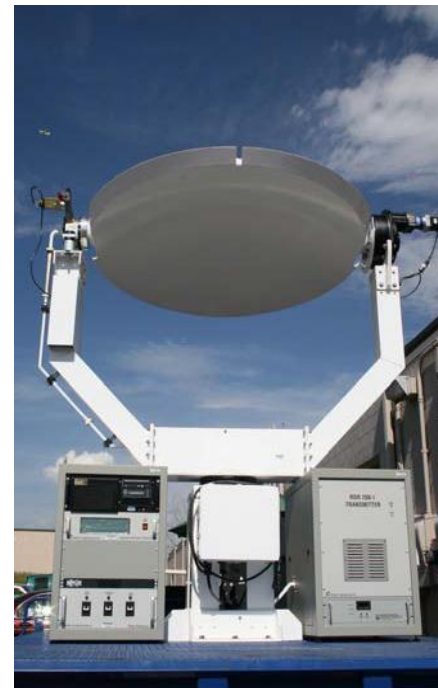
“Package” RDR-200GX System For Mounting Inside Radome
